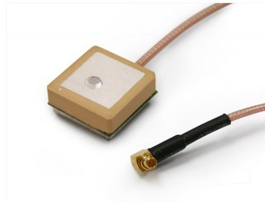
ADA-15S is a most compact/thin high gain GPS 3V and 5V antenna module. With comprehensive coverage almost all way to the horizon, it performs excellent in foliage or urban canyon environment. Also, ADA-15S is compatible with most GPS receives available on the market and provides a perfect alternative for the application of the GPS in different fields.
